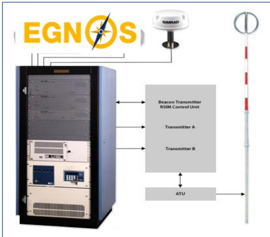
DGSS station: GNSS receiver + MF transmitter. Courtesy: MxMarine
